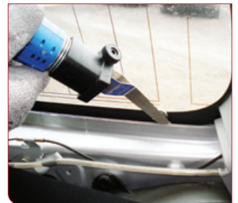
WK24ZV-S Serrated Offset V Blade - 150mm Long
